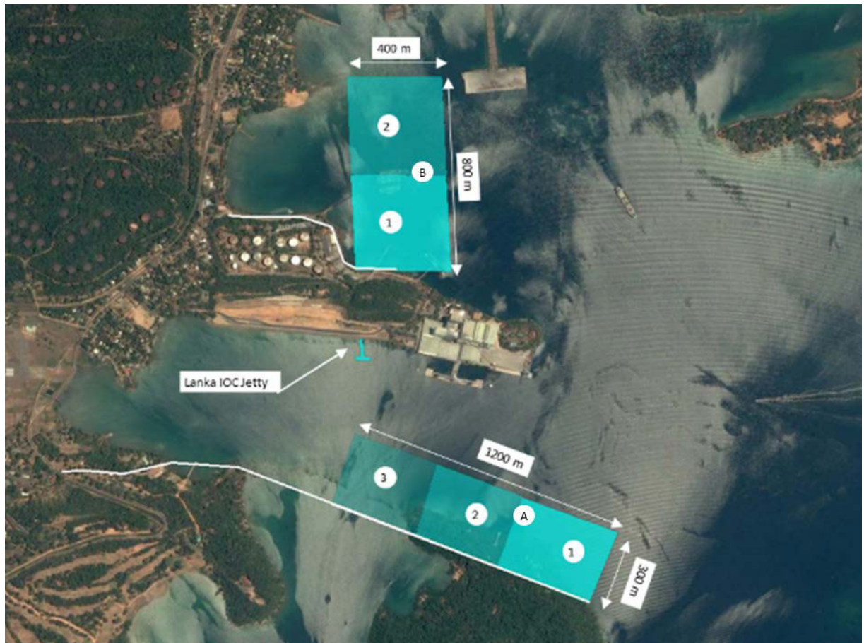
Figure 5-15: Two Options Accommodation Container Terminal
