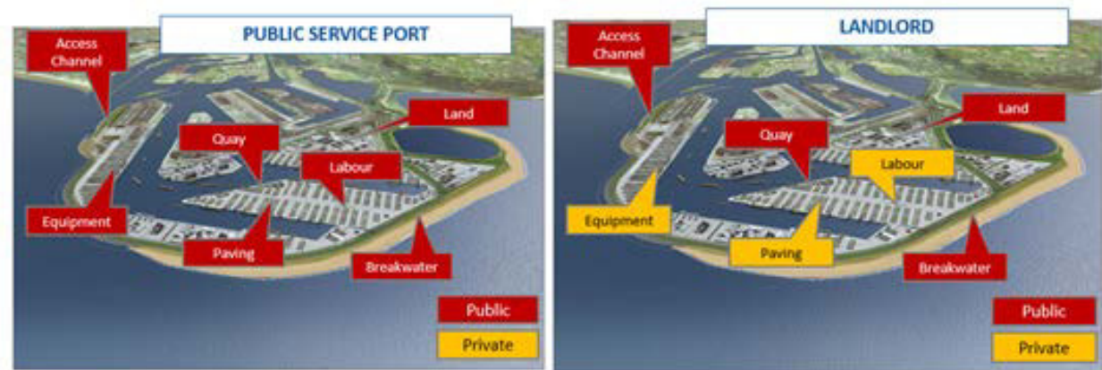
Figure 2-18 Public Service Port and Landlord Port model
